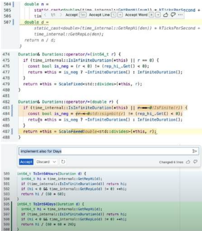
Fig. 3. A demonstration of how a variety of AI-based features can work together to assist with coding in the IDE. top: code completion, middle: adjusting copy-pasted code to the context, bottom: code edits based on natural language instructions. See our blog for more details [3].
